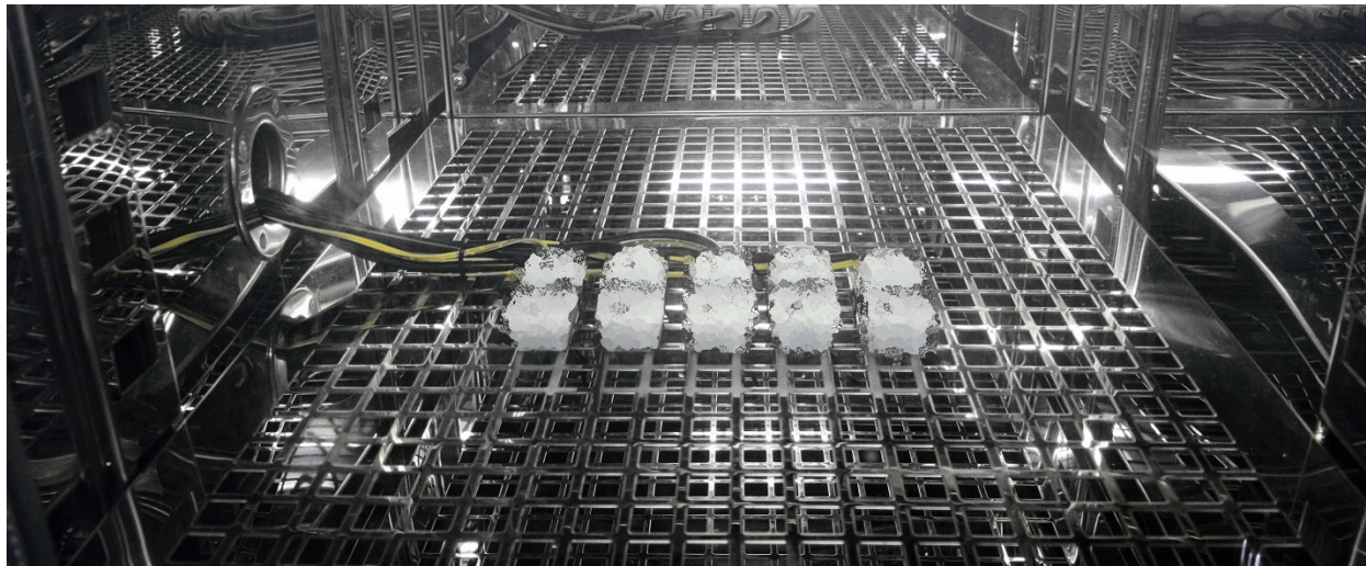
Figure 2: Switch-1es (SW-1) fixtured within an environmental chamber ("A"-"E", left to right)
