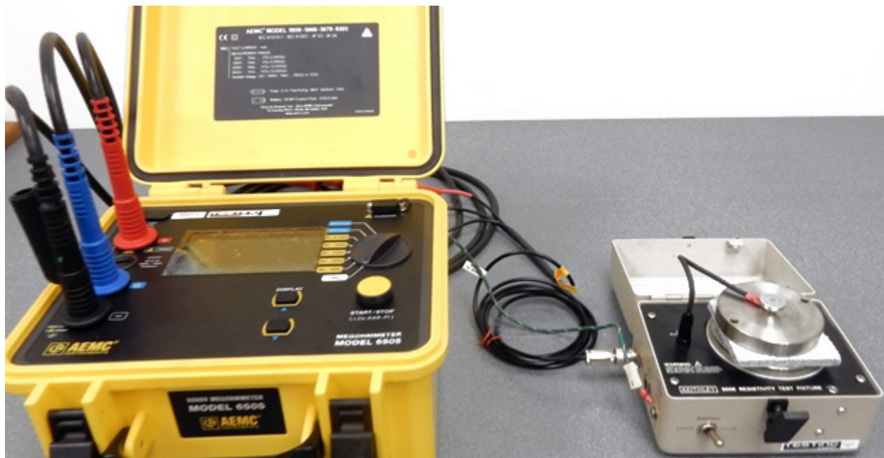
Figure 1: AEMC Megohmmeter and Keithley resistivity test fixture
