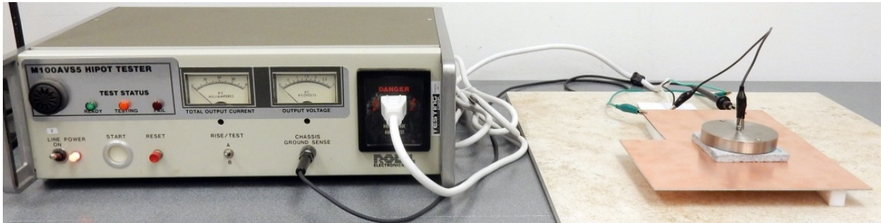
Figure 2: Hipot tester and test fixture
