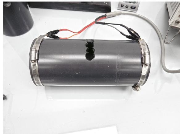
Figure 3: Transversely drilled pipe
