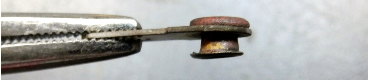
Figure 4: Fuse terminal and semi-tubular rivet
