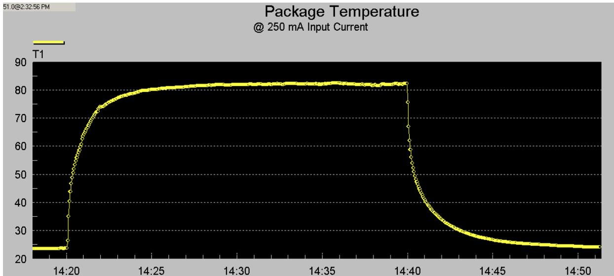
The following graph shows the temperature rise of the part when the input current dropped to 170 milliamperes due to disconnecting one pair of parallel-connected white LEDs (i.e., the output current was reduced to 80 milliamperes, reducing the internal power dissipation to 320 milliwatts and raising the power conversion efficiency to 53%). Note that the peak temperature only reached 69.7° C compared to a peak of 82.4° C when supplying 120 milliamperes.
