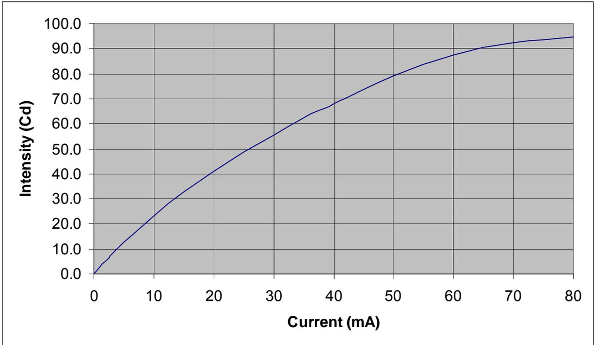
In the client's new-design, the white LEDs are each operating at 20 milliamperes (mA), and so, according to the chart, should be emitting about 40 candelas.
