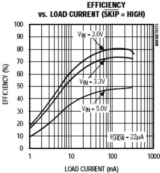
The high temperatures measured and plotted above turns out to be worst-case, because the part actually becomes MORE efficient as the battery voltage drops, as seen in this plot (right) taken from the part specification sheet:
