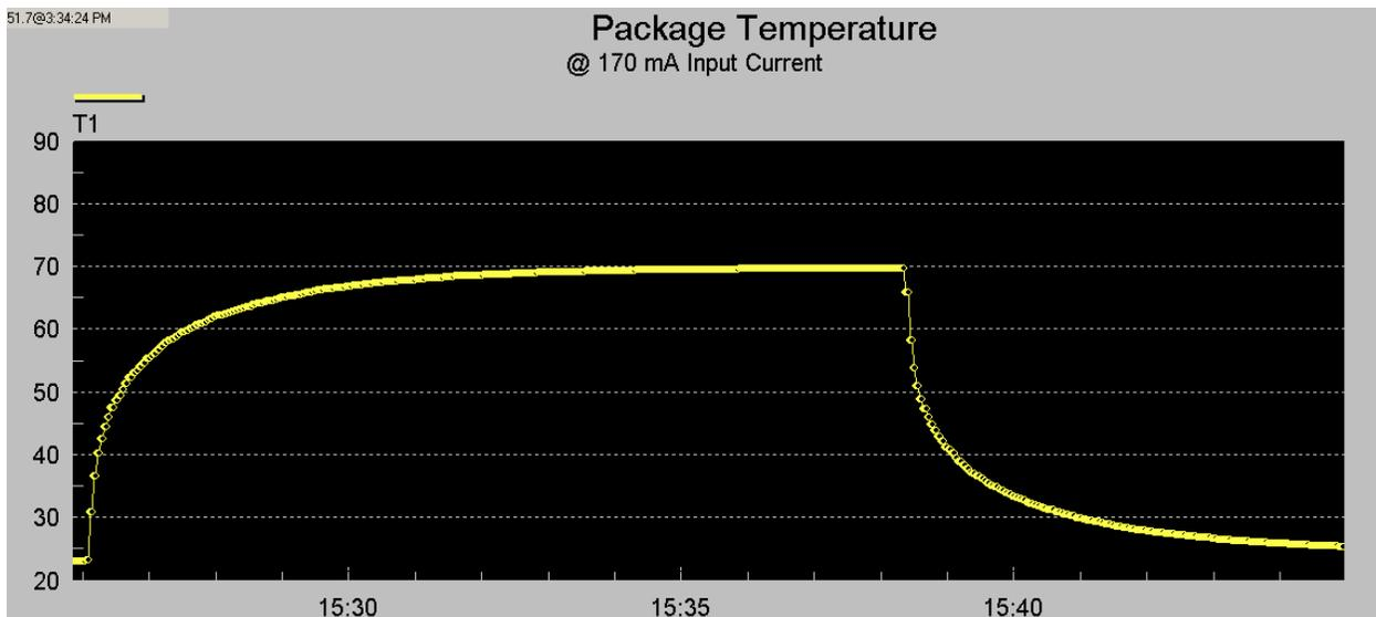
The case temperature can be predicted mathematically by noting that the thermal resistance of the part's SO-8 package is 160°C per watt.
